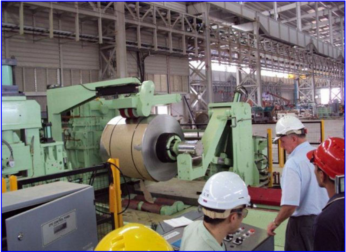
First coil processed in the slitting line
