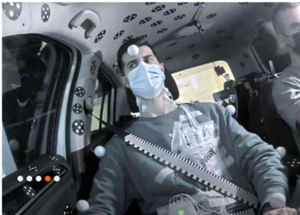
We have validated a set of procedures to better understand how vehicle occupants behave before an accident and to assess the impact of ADAS functions on their protection. We conduct tests on driving simulators and tracks, as well as human body model (HBM) simulations, which are key to understanding how active safety systems influence the performance of restraint systems and develop effective countermeasures for safer vehicles.
