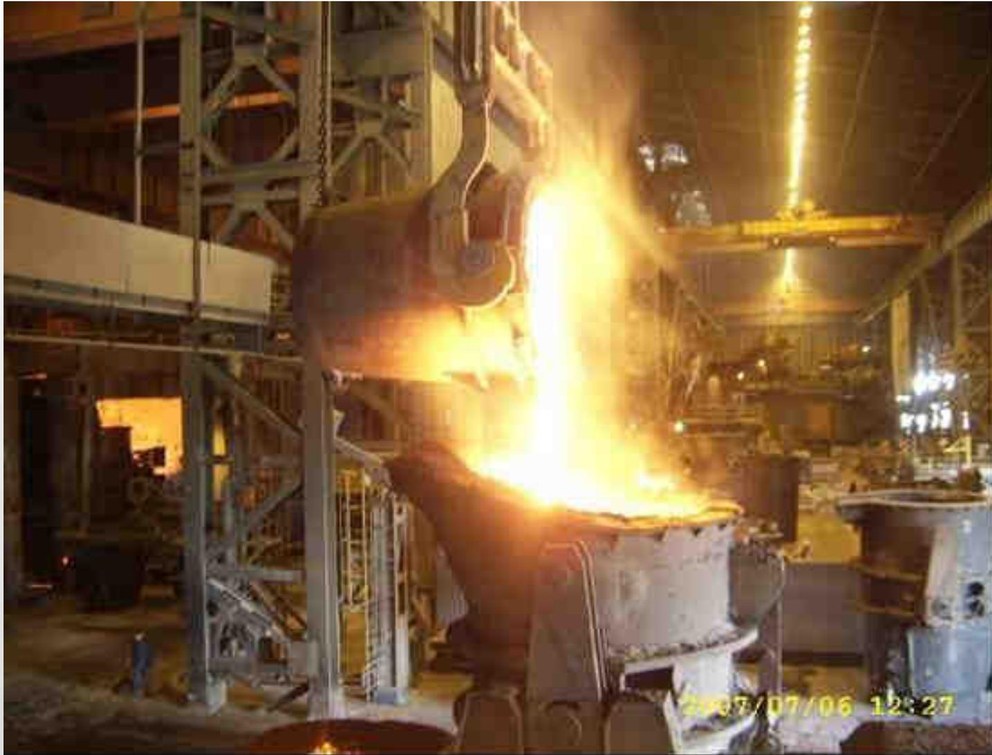
**Decanting of MFC ladle filled with Liquid ferrochrome into EAF transfer ladle**
