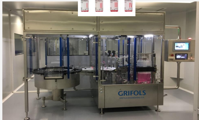
Automated red cells filling machine; Barcelona
