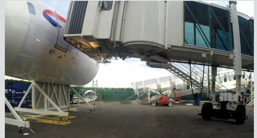
Autonomous passenger bridge trial
