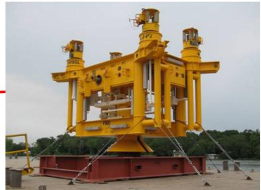
Gas Lift Distribution Unit (GLDU)
