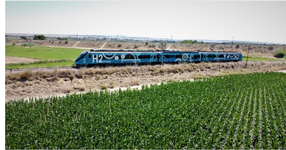
28/07/2022. On-track dynamic testing of the hydrogen train prototype of the FCH2Rail project, developed by the consortium of companies formed by CAF, DLR, Toyota, Renfe, ADIF, CNH2 and Stemmann-Technik.
