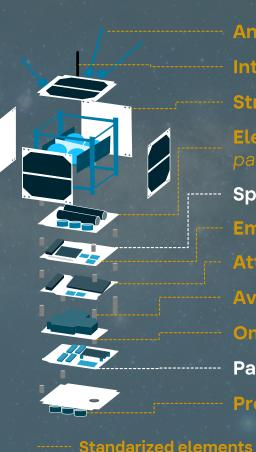
Illustrative LEO satellite Antennas Inter-satellite Link Structure and Thermal Subsystem Electric and Power system (e.q. solar **Specialized Software** (e.q. military) **Embedded Software** Attitude and Orbit Control System **Avionics On-board computer Payload** (e.q. radar, comms., optical) Propulsion
